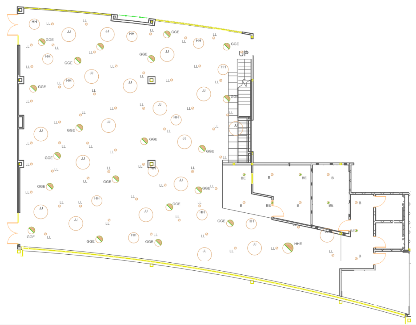
Figure 5: Reflected Ceiling Plan of Existing Lighting in Media Center
